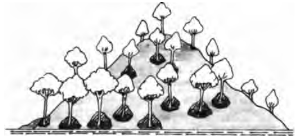
Fig 12. Individual "eyebrow" terraces. Accommodate only one tree but are very useful to control erosion at a relatively low cost.
