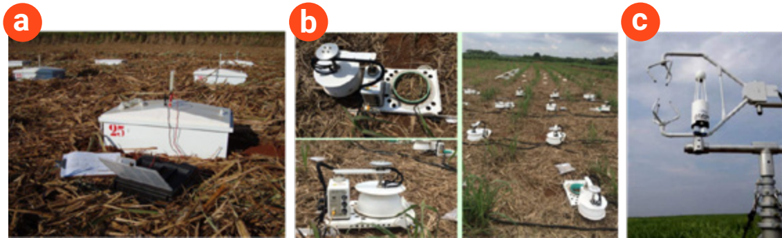
Figure 4. Methodologies used for sampling greenhouse gases emitted from the soil in the field. a) static chambers; b) dynamic chambers, c) tower of eddy covariance.
