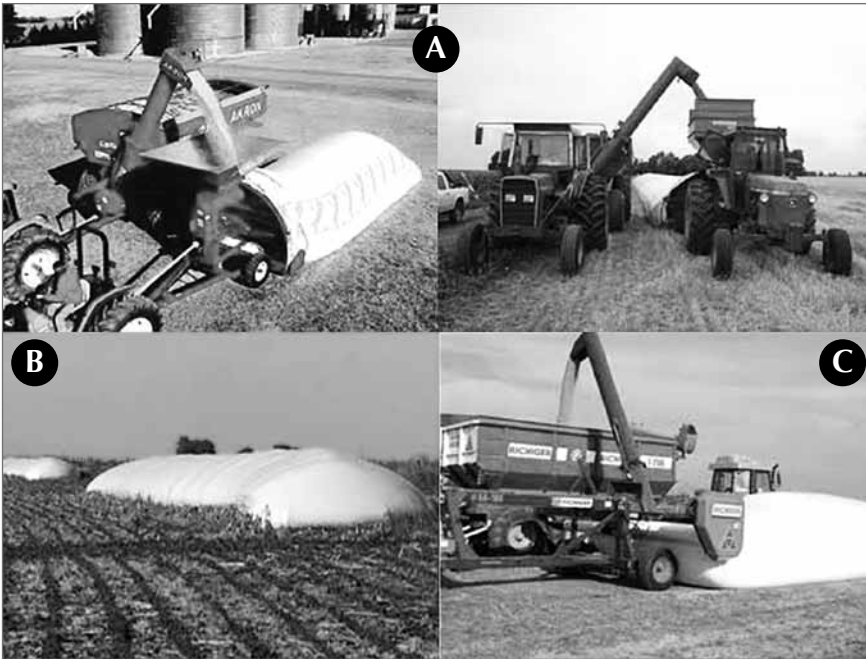
Figure 2.4. Silo bag system: (A) building of the silo, (B) silo bag completed and (C) extraction of the grain from the silo
