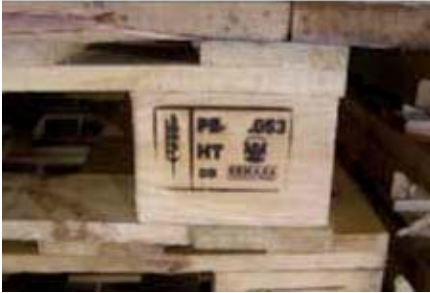
Pallet stamped with ISPM 15 compliance seal
