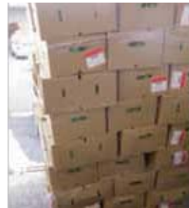
Boxes stowed in crisscross pattern collapsed by the weight on
